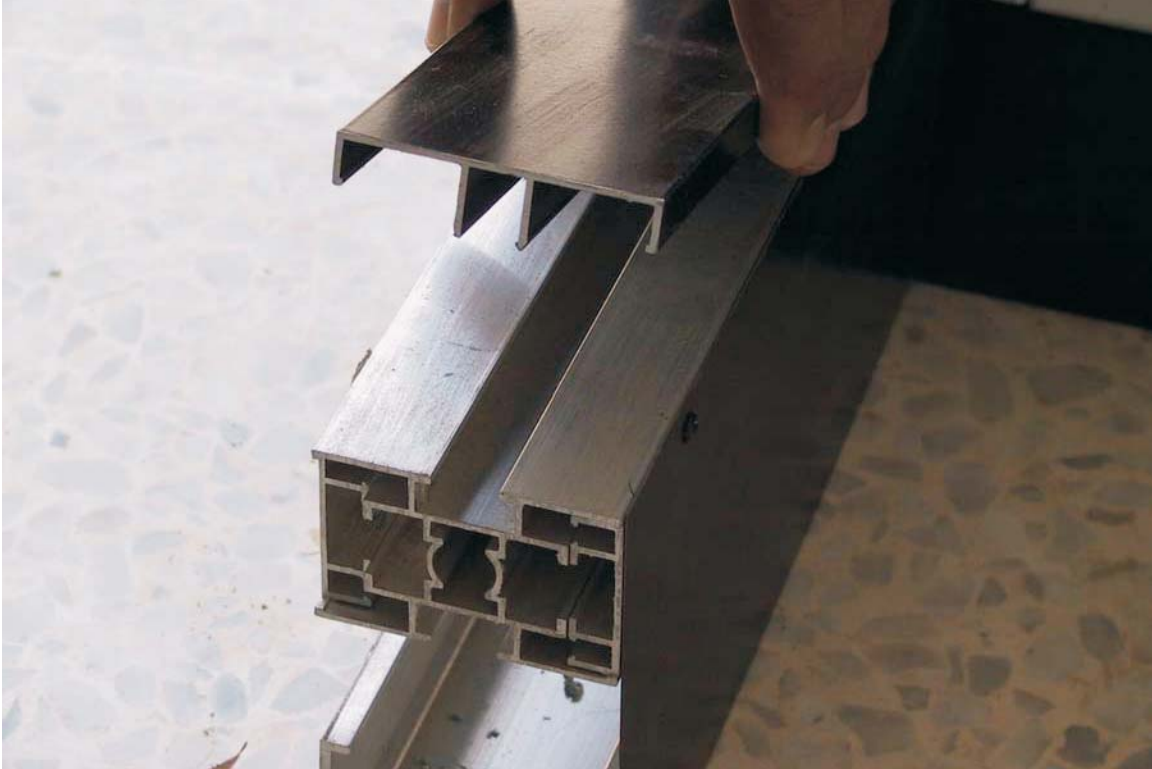
Internal Structure cover installation.
